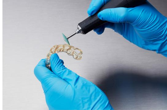
**Note:** Remove supports only after post-curing to ensure that parts do not warp.
